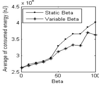
Fig. 11: Changes in average consumed energy by adopting type I path cost equation in case of single sink network with respect to static
