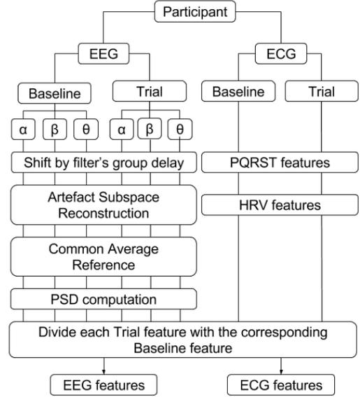
Fig. 4. Outline of the feature extraction procedure.
