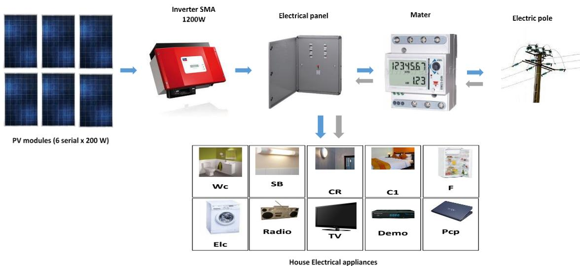
Figure 5. The general scheme of the proposed grid-connected PV system
