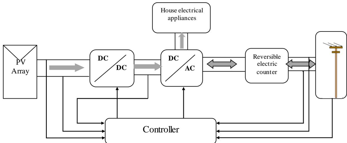
Figure 4. Block diagram of the grid connected photovoltaic system
