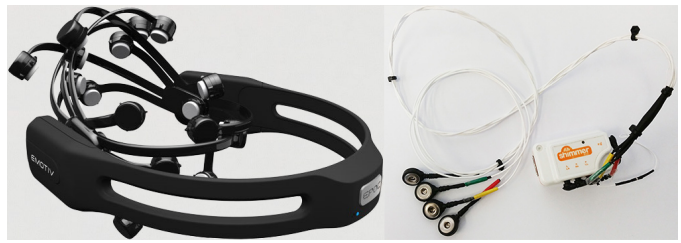
Fig. 1. The Emotiv EPOC wireless EEG headset and the wireless SHIMMER ECG sensor.
