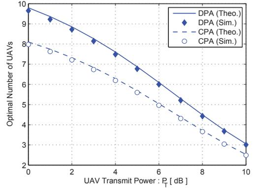
Fig. 4: Number of the needed UAVs vs.  $P_T$ , with  $\lambda_p = 3e - 6$  m<sup>-2</sup>.
