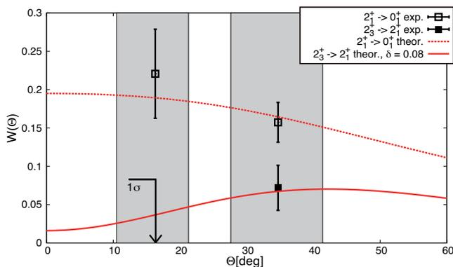
FIG. 4. (color online) Observed intensities with their statistical uncertainties (data points) and calculated angular distributions for the  $2_1^+ \rightarrow 0_1^+$  with pure  $E2$  character (dashed line) and the  $2_3^+ \rightarrow 2_1^+$  (solid line) transitions. The angular range of the inner and outer ring of germanium detectors are marked with gray color. A  $1\sigma$  observation limit is indicated for the  $2_3^+ \rightarrow 2_1^+$  in the inner ring.
