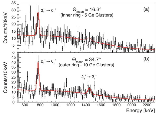
FIG. 3. (color online) Doppler corrected  $\gamma$ -ray energy spectra for  $^{88}\text{Kr}$  for the inner (a) and outer (b) ring of germanium detectors in the PreSPEC setup. The spectra are drawn with their statistical errors. Fits to the observed transitions and the  $1\sigma$  observation limit in case of the  $2_3^+ \rightarrow 2_1^+$  in the inner ring and a background function are indicated with the red (gray) line (see text for details).
