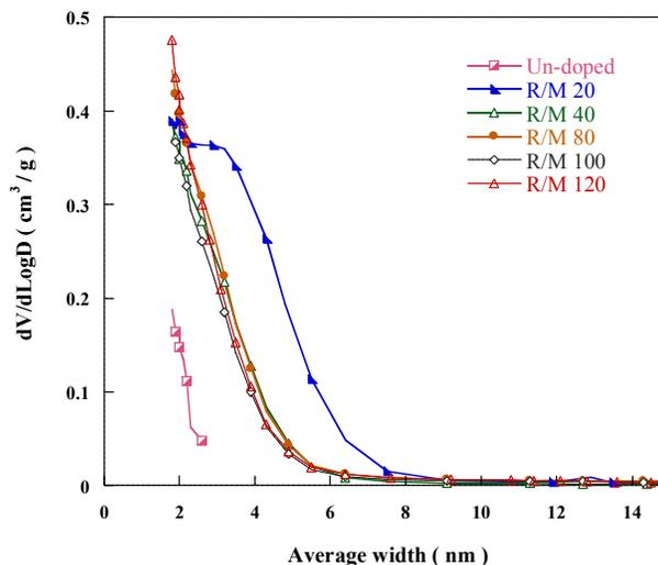
**Figure 2** Pore size distribution of un-doped and nitrogen doped (different R/M ratios) carbon aerogels.
