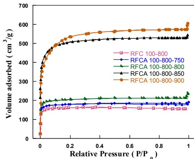
**Figure 5** – N<sub>2</sub> adsorption–desorption isotherms of carbon / activated carbon aerogels.
