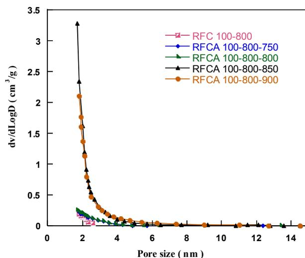
**Figure 6** – Pore size distribution of carbon/activated carbon aerogels.
