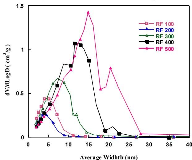
**Figure 2** Pore size distribution of RF aerogels with different R/C ratios.
