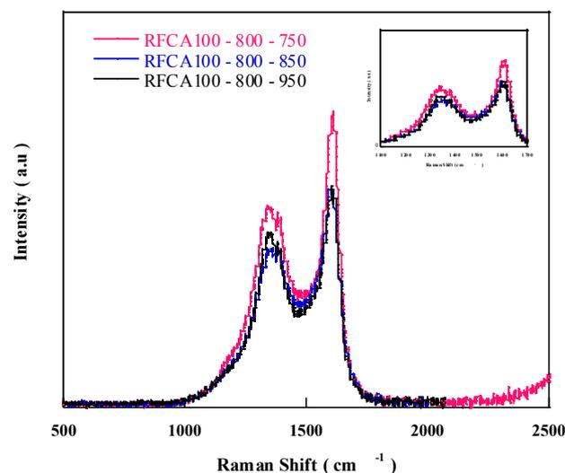
**Figure 7** Raman spectra of RFCA 100-800 activated at different temperatures.
