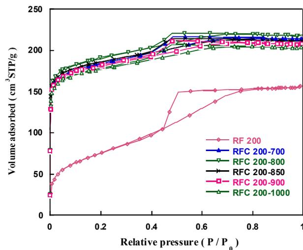
**Figure 3** N<sub>2</sub> adsorption–desorption isotherms of carbon aerogels produced at different temperatures.
