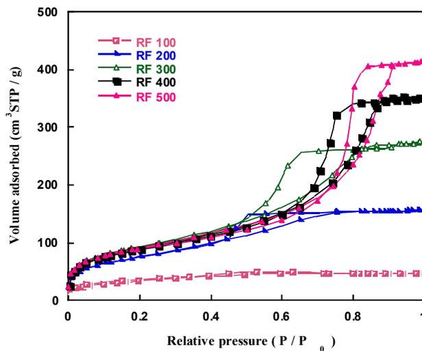
**Figure 1** N<sub>2</sub> adsorption–desorption isotherms of R/F aerogels with different R/C ratios.
