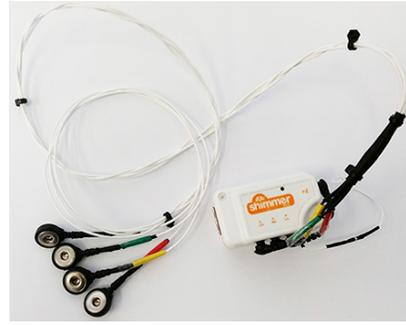
Fig. 1: The SHIMMER™ v2.0 wireless ECG sensor
