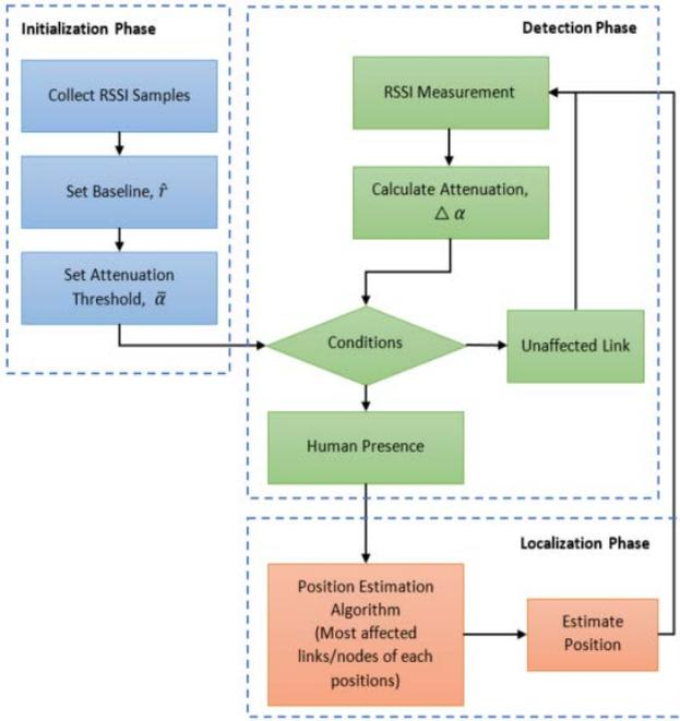
Fig. 1. The deterministic algorithm of a DFL system.
