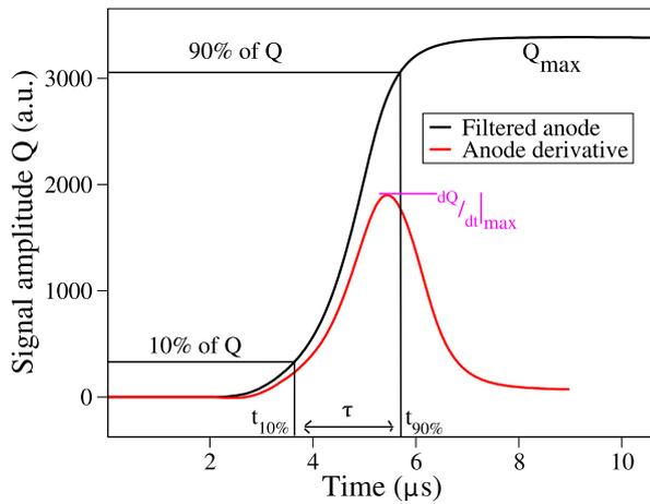
Fig. 4. A typical anode signal averaged over > 1000 FF shown with its derivative in red. The derivative has been shifted right and scaled for clarity. The parameters of interest corresponding to maximum energy, maximum energy loss, and 10% to 90% risetime are shown. (For interpretation of the references to colour in this figure legend, the reader is referred to the web version of this article.)
