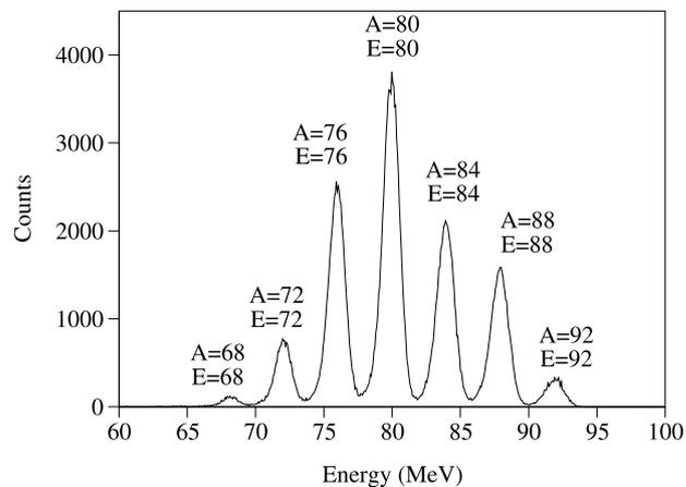
Fig. 3. A typical energy spectrum extracted from the filtered and corrected anode signals for Lohengrin settings  $A = 80$  amu,  $q = 20$ ,  $E = 80$  MeV. The peaks in the spectrum are indicated with their corresponding mass and are clearly separated from each other. Each of the mass peaks contains contributions from several different isobars.
