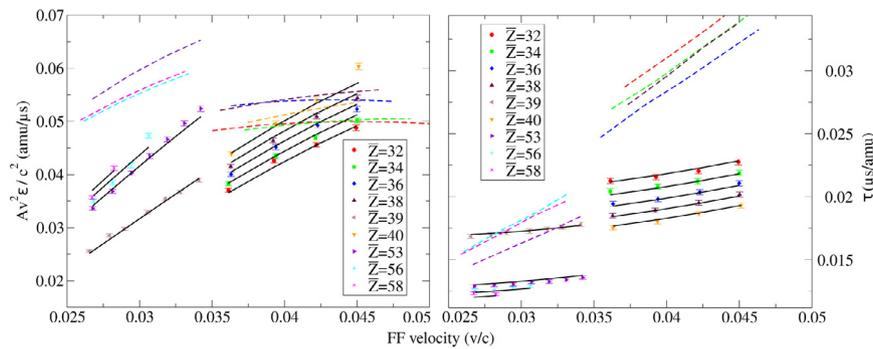
Fig. 5. Plots of  $A(\frac{v}{c})^2\epsilon$  against FF velocity on the left and  $\tau$  against velocity on the right. Lines corresponding to separate values of FF  $Z$  are easily distinguishable in both plots. There are two clusters present: one for heavy and one for light fragments. Functional fits to the parameters are in solid lines and results of a SRIM-2013 simulation for the same fragments are in dashed lines. See text for details.
