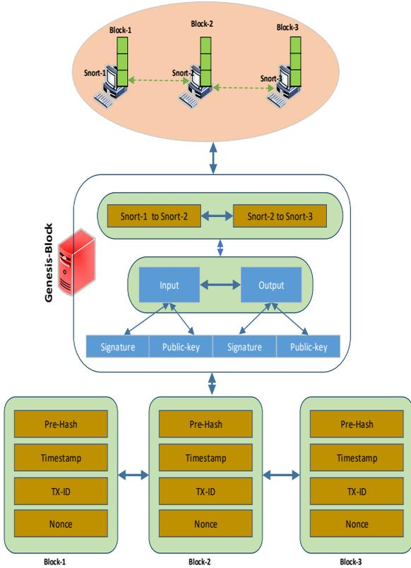
Fig. 2. Blockchain trust communication inside CIDN Snort nodes.
