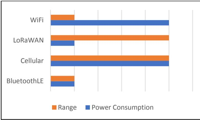
Figure 2 - Range vs Power Consumption (adapted from [20])
