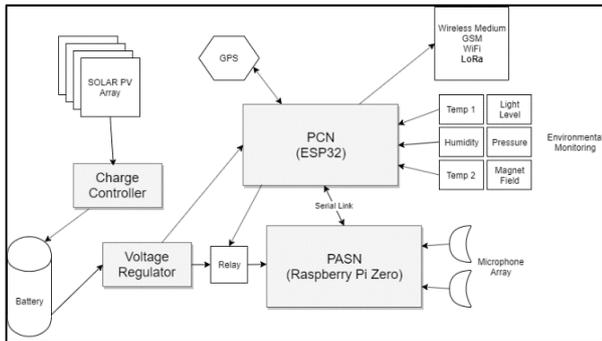
Figure 1 - Block diagram of the PANDI System.
