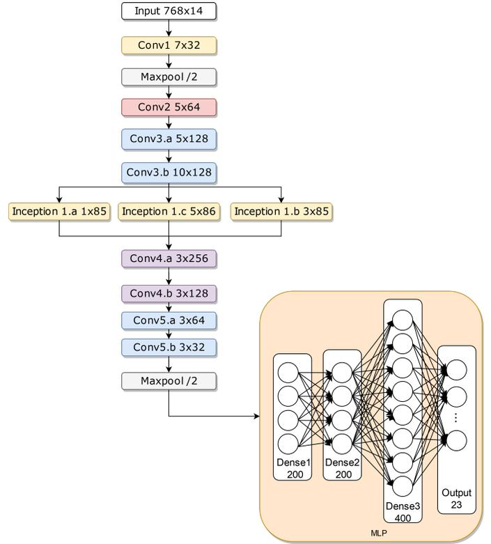
Fig. 1. Proposed network architecture for EEG-based subject identification
