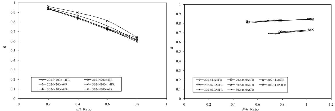
Fig. 3: Variation in reduction factors with  $a/h$  and  $N/h$  for under ITF loading condition
