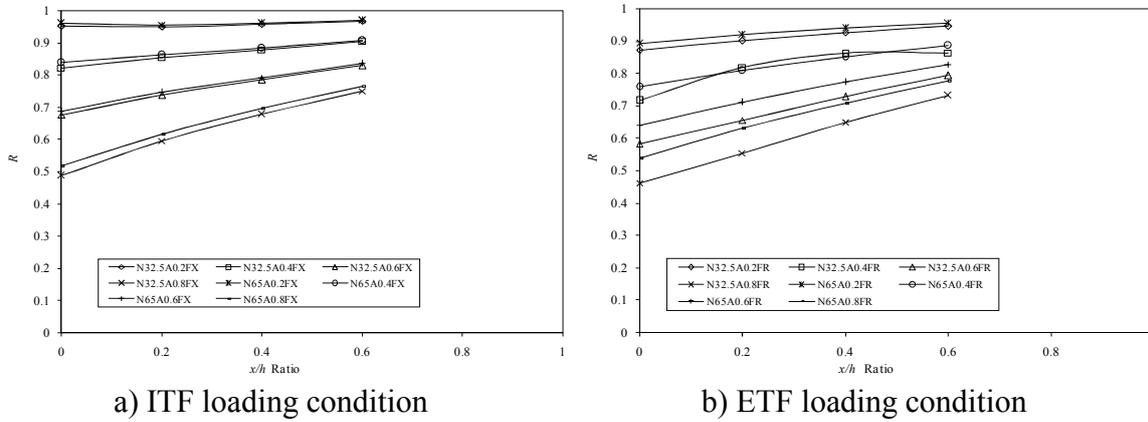
Fig. 2: Variation in reduction factors with  $x/h$  ratio
