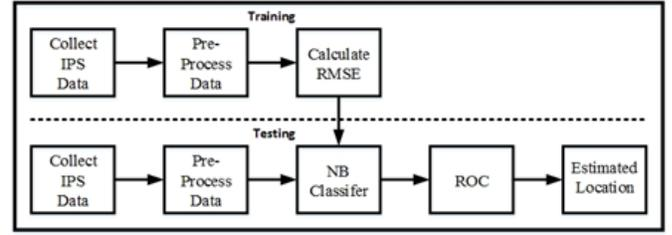
Fig. 1. Block Diagram of developed UWB IPS system
