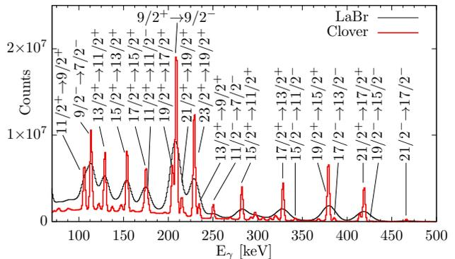
Figure 1. (Color online) Full projections of the clover (red) and LaBr<sub>3</sub> (black) threefold coincidences measured during the 72 h measurement. The clover (LaBr<sub>3</sub>) spectrum is generated by using Ge-LaBr<sub>3</sub>-Ge (Ge-LaBr<sub>3</sub>-LaBr<sub>3</sub>) events, respectively. The dominant transitions in <sup>177</sup>Hf are labeled.
