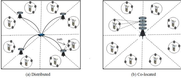
Fig. 1. Distributed and co-located mm-Wave massive MU-MIMO systems.
