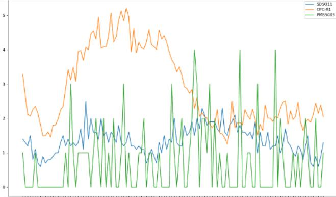
Figure 2: Comparison plot of PM sensors (SDS011: Blue, OPC-R1: Orange and PMS5003: Green) in a controlled lab environment (no human or any other mobility within the environment) for  $PM_{2.5}$  for 48 hours where the linearity of the plot is analysed as one of the sensor selection criteria.
