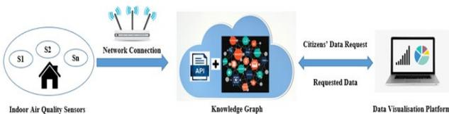
Figure 1: Indoor Air Quality Monitoring: System Architecture
