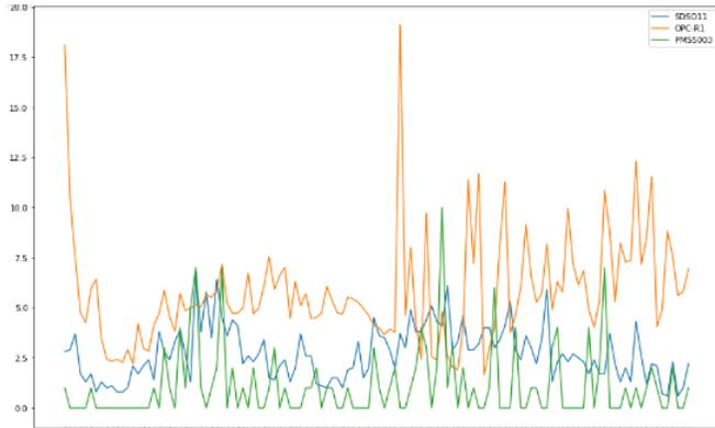
Figure 3: Comparison plot of PM sensors (SDS011: Blue, OPC-R1: Orange and PMS5003: Green) in a controlled lab environment (no human or any other mobility within the environment) for  $PM_{10}$  for 48 hours where the linearity of the plot is analysed as one of the sensors selections criteria.
