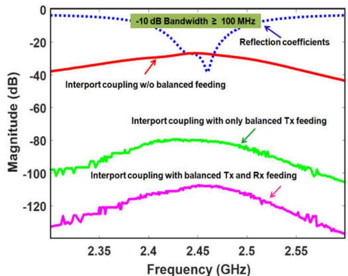
Fig. 3. The simulated reflection-coefficients and interport coupling levels for presented antenna with balanced  $T_x$  and  $R_x$  feeding.
