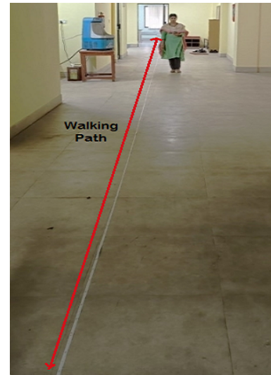
Fig. 7. Linear path walked by some participant with smartphone in handheld mode in experimental site.
