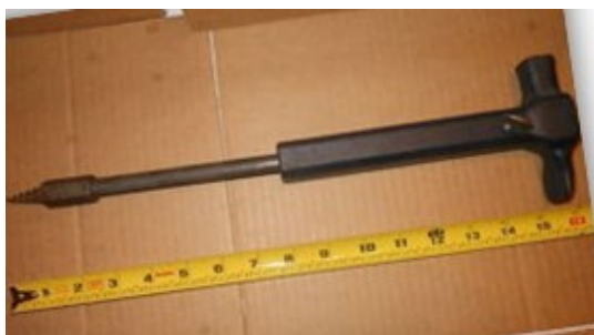
Fig. 2. Bung removal tool.
