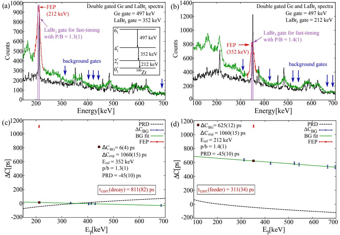
FIG. 5. Lifetime analysis for the  $2_1^+$  state in  $^{100}\text{Zr}$ . Panels a) and b) show the double-gated Ge (shown in black) and  $\text{LaBr}_3$  (green/gray) spectra. Panels c) and d) display the Compton background correction procedure (see text for details).
