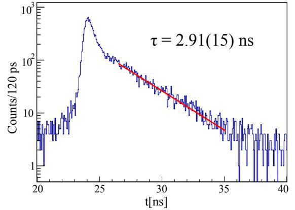
FIG. 6. Lifetime determination for the  $2_1^+$  state of  $^{102}\text{Zr}$  using the  $^{241}\text{Pu}$  target data. The independent anti-delayed time spectrum resulting from the FEP events is inverted and aligned before being summed to the delayed time distribution. The slope has been determined by fitting the data in the range from 25.5 ns to 35 ns.
