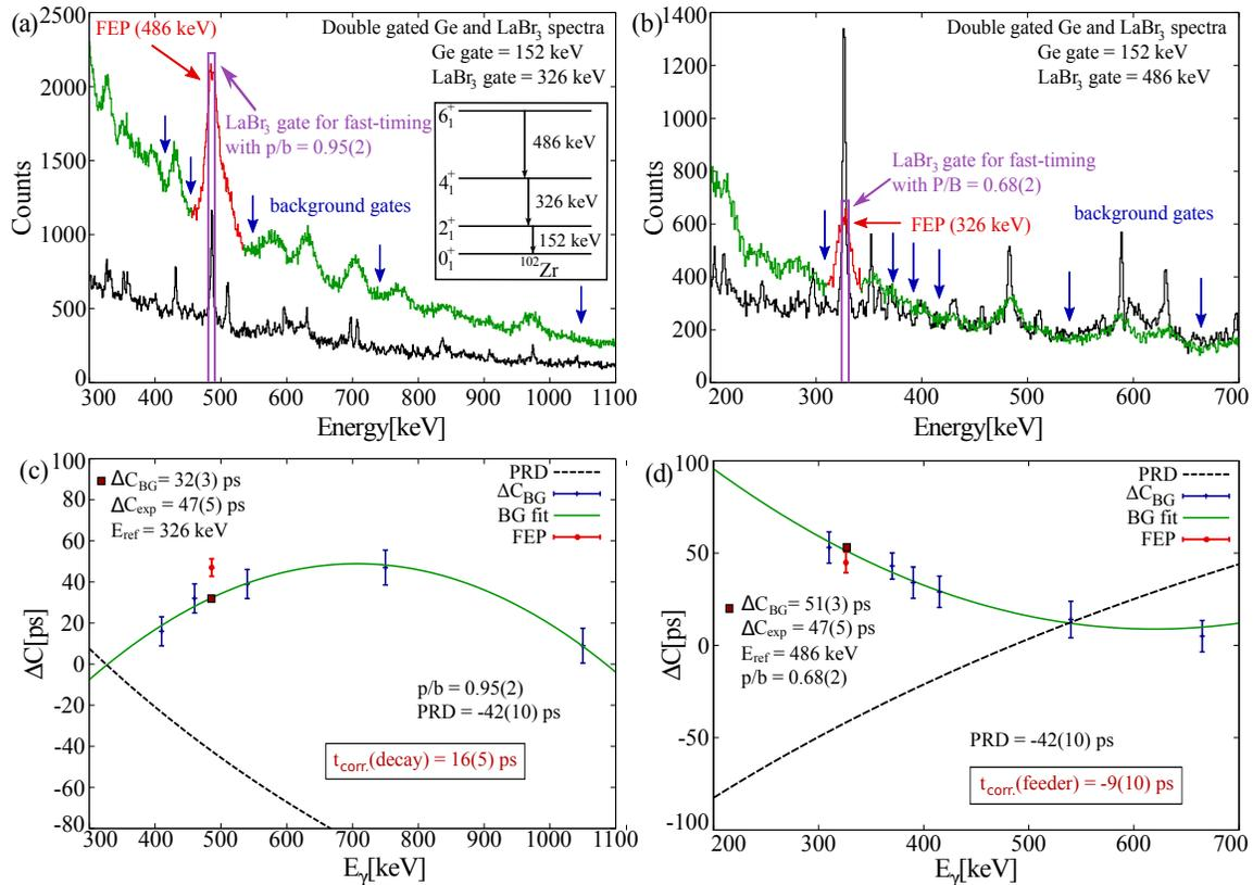
FIG. 7. Lifetime analysis for the  $4_1^+$  state in  $^{102}\text{Zr}$ . Panels a) and b) display double-gated Ge (shown in black) and  $\text{LaBr}_3$  (green/light gray) spectra. Panels c) and d) show the Compton background correction procedure (see text for details).
