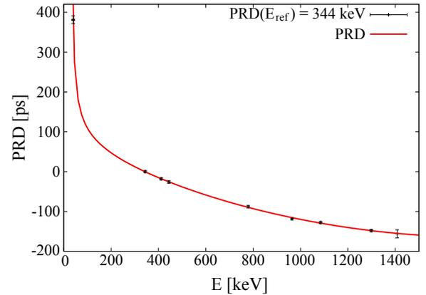
FIG. 2. PRD curve obtained using a  $^{152}\text{Eu}$  source.
