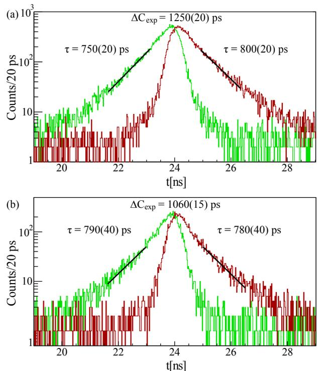
FIG. 4. Lifetime determination using the slope method for the  $2_1^+$  state of  $^{100}\text{Zr}$ . (a) displays the delayed (red) and the anti-delayed (green/light gray) time distributions of the state of interest from  $^{235}\text{U}$  fission, and (b) from  $^{241}\text{Pu}$  fission.
