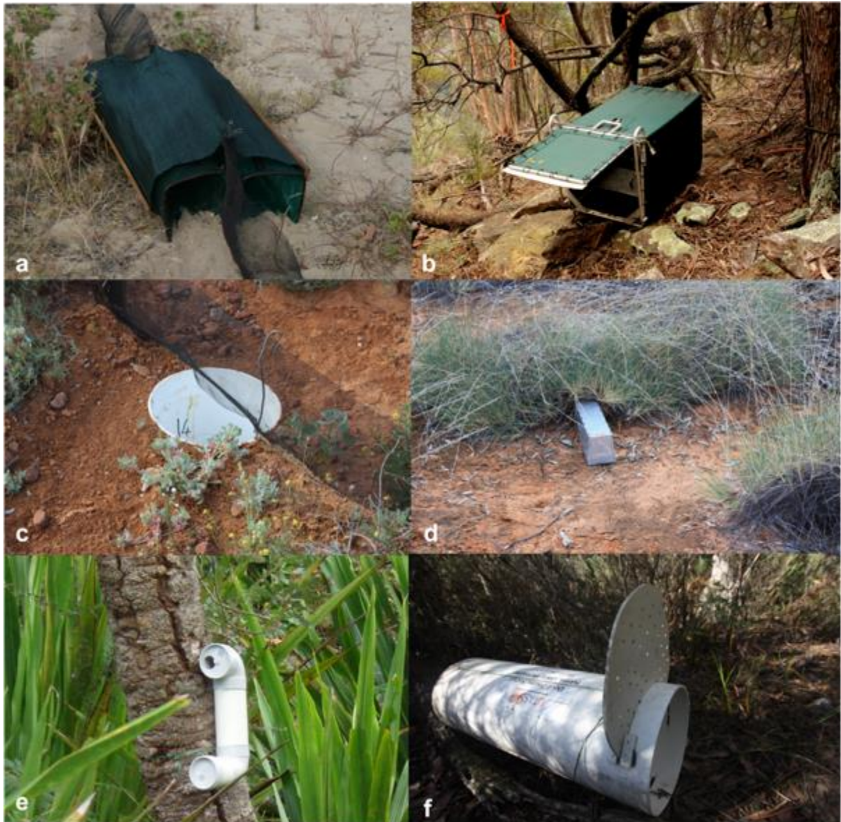
Figure 7.1. a) funnel traps with shade covers positioned alongside drift-net fencing (photo by Terrestrial Ecosystems); b) soft-sided cage trap often used for wallaby capture (photo by David Taggart); c) Elliott trap placed near vegetative shelter (photo by Helen P. Waudby); d) pitfall trap for capturing ground-dwelling fauna (photo by Helen P. Waudby); e) arboreal pipe trap (photo by James M. Turner); f) ground-based pipe trap for catching large dasyurids (photo by David Hamilton).
