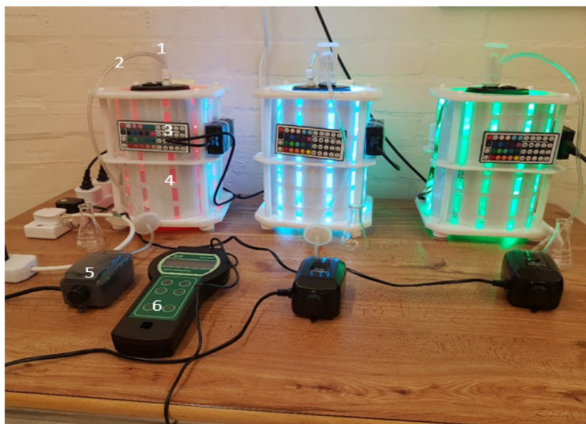
Figure 1. Closed PBR used in this research. (1) Tube head; (2) \text{CO}_2 tube; (3) LED lighting remote; (4) PBR outer cover; (5) pump for mixing; (6) handheld photometer.
