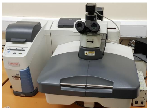
Figure 1: Thermo Scientific DXR Raman Microscope
