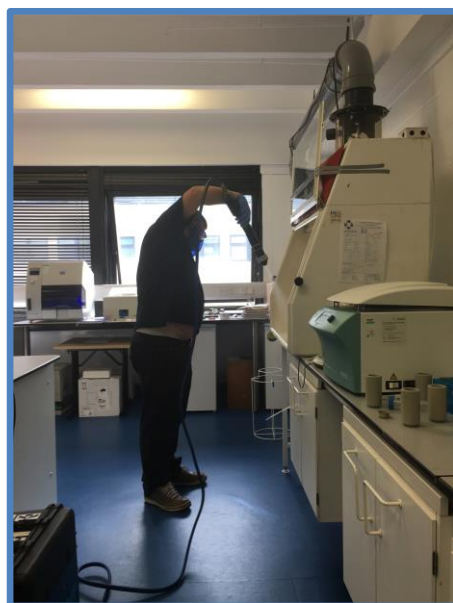
Figure 2: Operational setup used for the H 2 O 2 electrostatic spraying (SanoStatic) experiments
