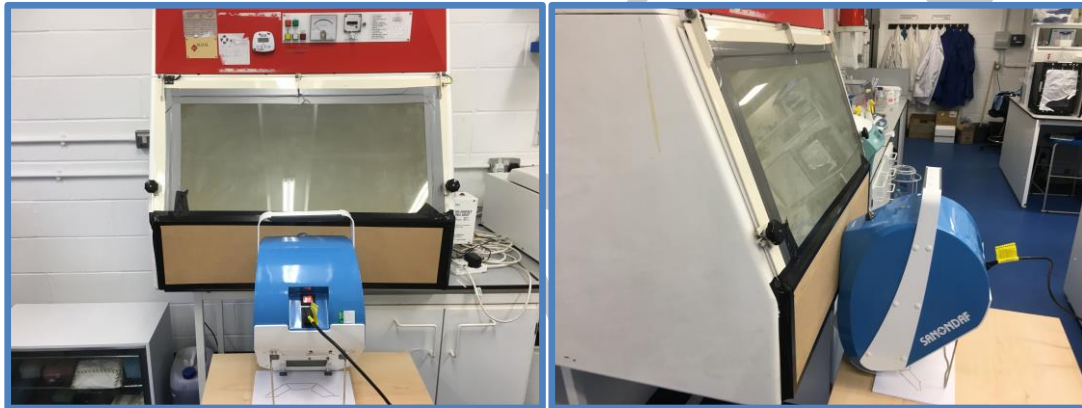
Figure 1: Operational setup used for the H 2 O 2 fogging (SanoFog) experiments
