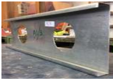
(a) Section with unstiffened holes
